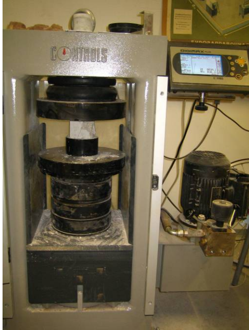
Figure 1 Press for uniaxial compressive strength tests
