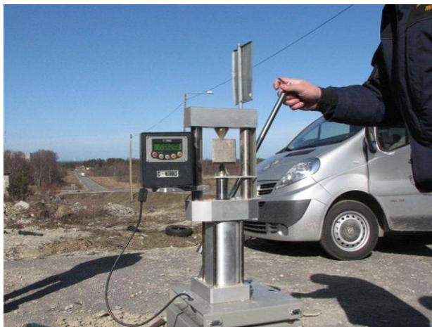
Figure 12 Point load test
