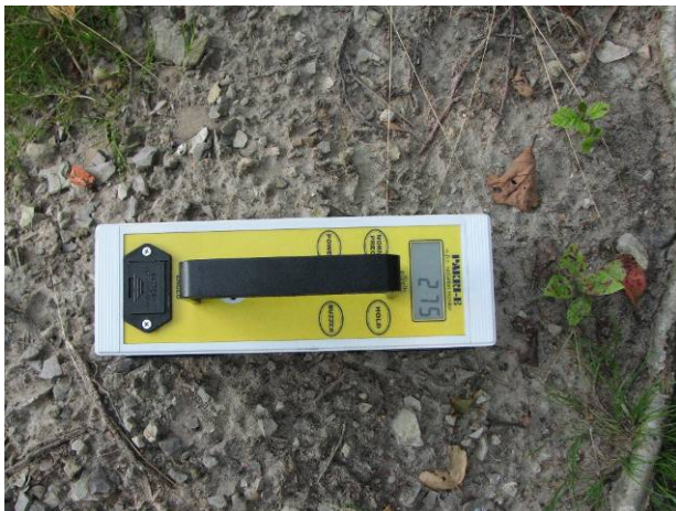
Figure 20 Radioactive radiation meter Pakri-E
