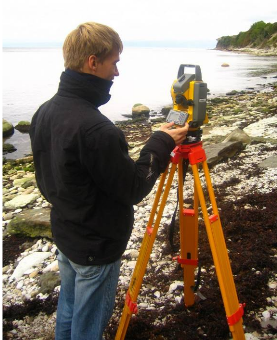
Figure 26 Tachymeter Trimble M3 Total Station
