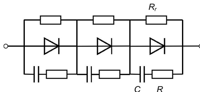
Figure 4.6. Equalization of power semiconductor voltages on serial connection
