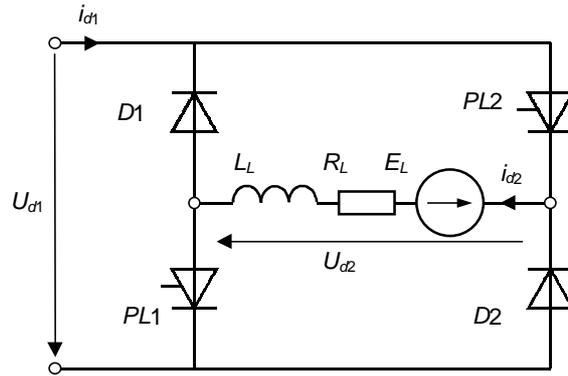
Figure 4.20. Two-quadrant, variable output voltage polarity DC converter
