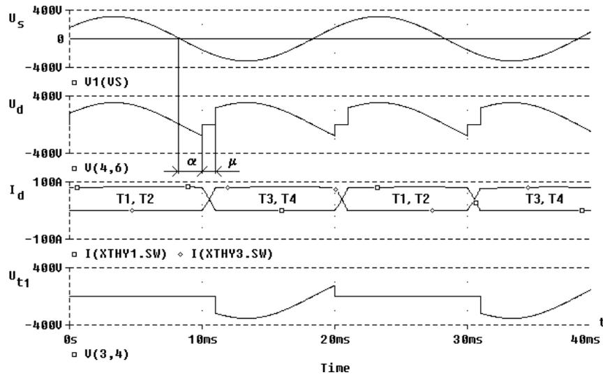
Figure 4.13. Voltage and current waveforms of the single-phase bridge rectifier B2 on ideal current smoothing, control angle  $\alpha = 30^\circ$  and commutation angle  $\mu = 15^\circ$ .
