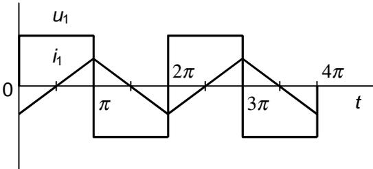
Figure 4.25. The waveforms of the output voltage and current on block controlled inverter.
