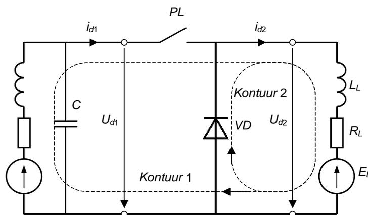
Figure 4.16. One-quadrant step-down (buck) DC pulse width converter together with supply and load circuits (for example motor)
