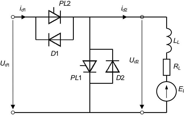
Figure 4.19. Two-quadrant, variable current direction DC converter
