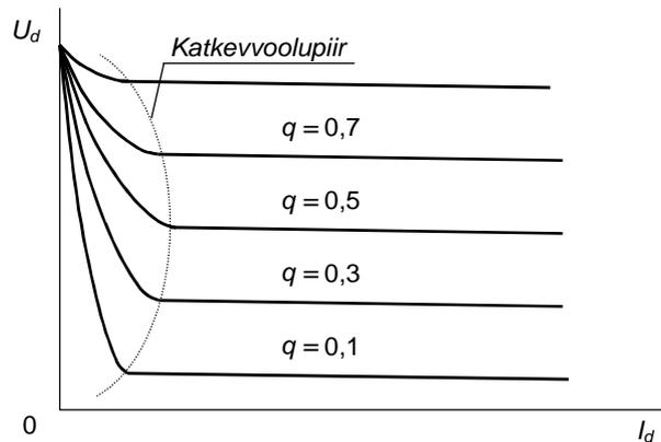
Figure 4.17. Output characteristics of step-down DC converter
