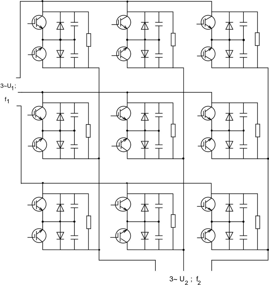
Figure 4.33. Power circuit diagram of the matrix converter
