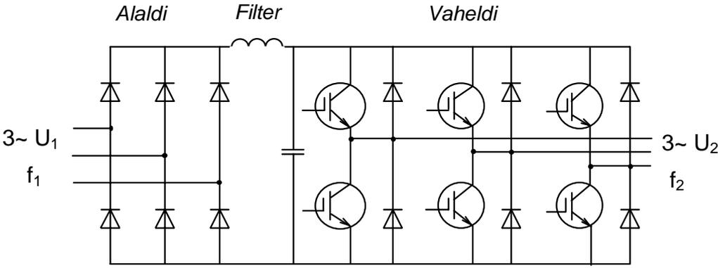
Figure 4.29. Power circuit diagram of Frequency converter with uncontrolled diode rectifier and transistor inverter
