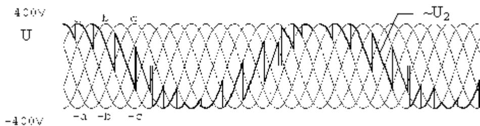
Figure 4.32. Output voltage waveform of the single-phase cycloconverter
