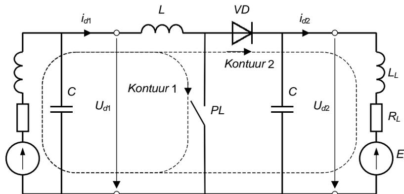
Figure 4.18. Step-up (boost) DC converter
