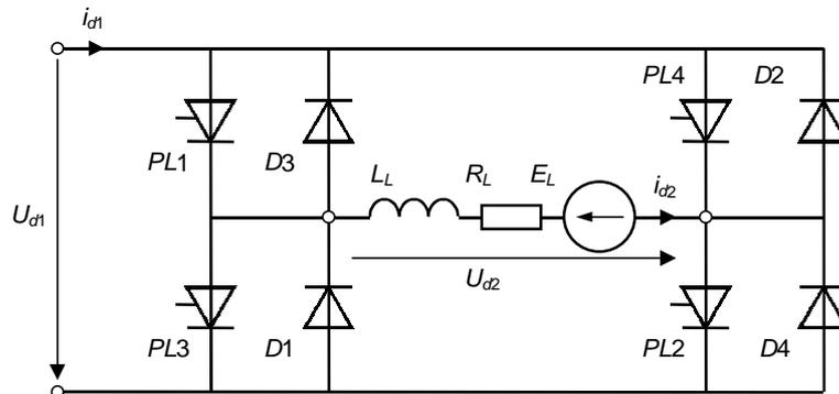
Figure 4.21. Four-quadrant DC converter
