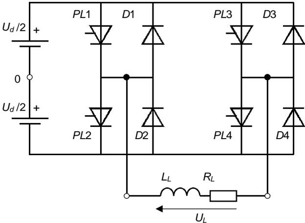
Figure 4.24. Offline inverter based on single-phase bridge circuit
