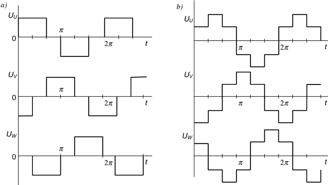
Figure 4.27. Output voltages of six-pulse three-phase inverter with block-control: a) By two simultaneously open switches, b) by three simultaneously open switches
