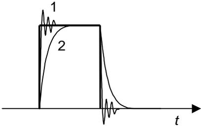
Figure 4.3. Switching transients and ringing effects
