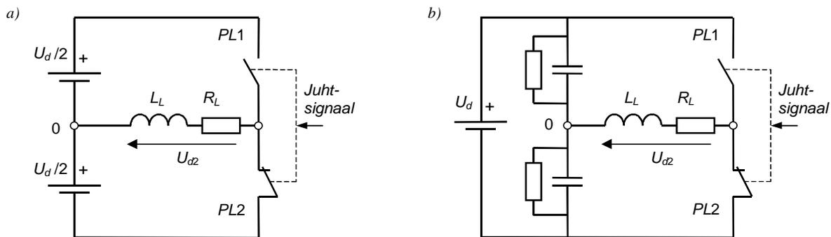
Figure 4.22. Inverter circuit diagrams: a) with two symmetrical supply sources, b) with voltage divider (artificial middle point)
