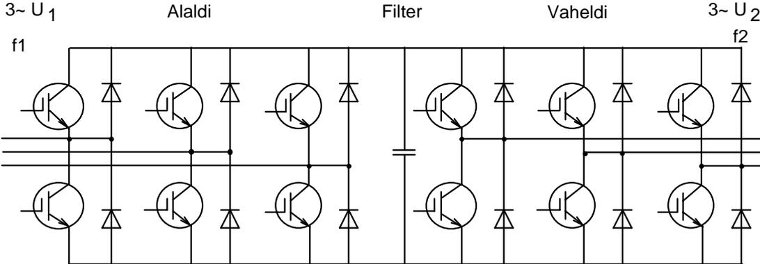
Figure 4.30. The power circuit diagram of the pulse width frequency converter with transistor rectifier and inverter
