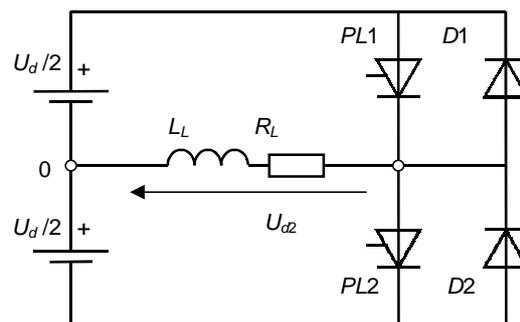
Figure 4.23. The circuit diagram of an offline half-bridge inverter with power thyristors and freewheeling diodes
