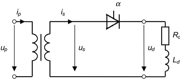
Figure 4.7. Single phase half period rectifier
