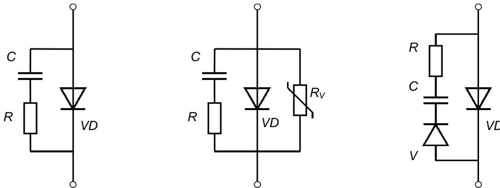
Figure 4.5. Over-voltage dumping circuits of the semiconductor switches:
