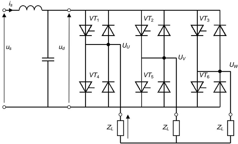
Figure 4.26. Three phase offline voltage inverter
