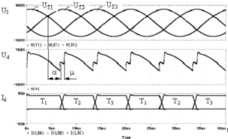
Figure 4.11. Voltage and current waveforms of three phase mid-point rectifier M3 on inductive load when the control angle  $\alpha = 45^\circ$  and commutation angle  $\mu = 15^\circ$ .
