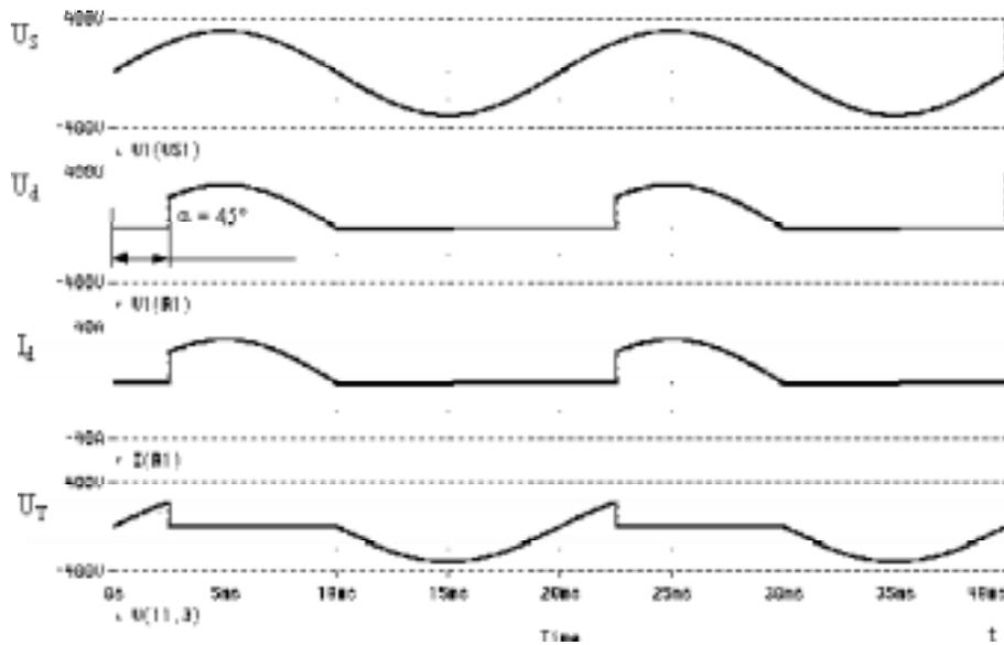
Figure 4.8. Current and voltage diagrams of the controlled half-period rectifier M1 on active load ( $L_d = 0$ ) with control angle  $\alpha = 45^\circ$ .
