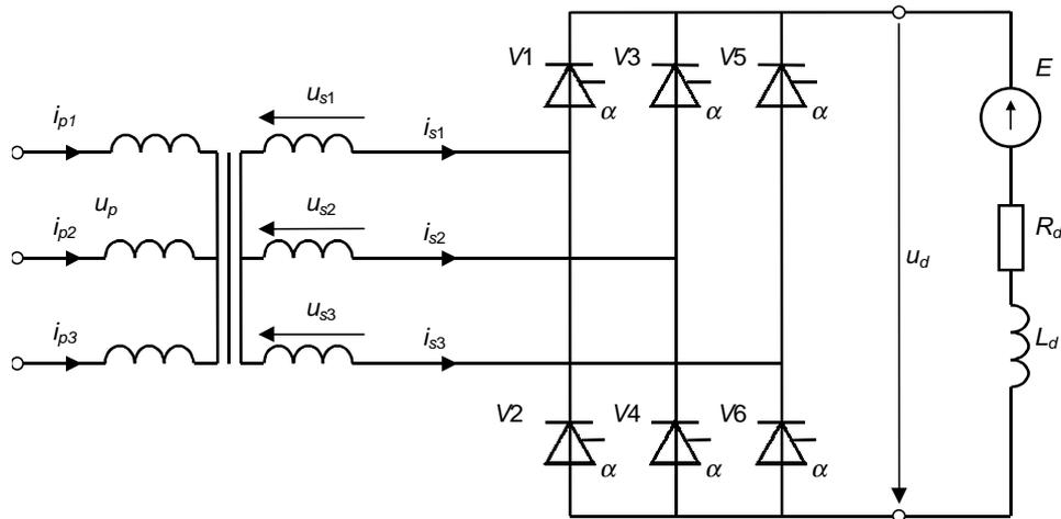
Figure 4.14 Three-phase bridge rectifier (B6)
