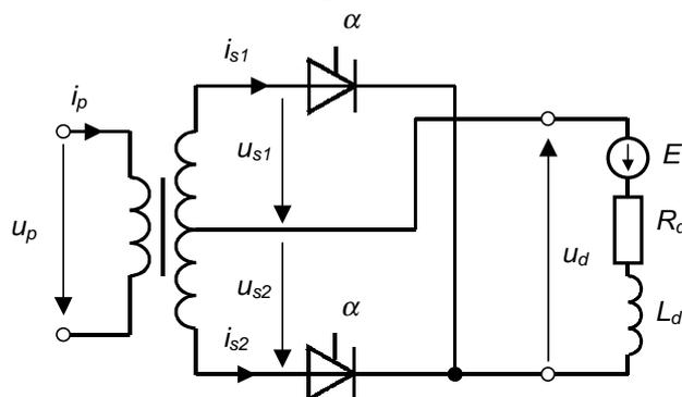
Figure 4.9. Single phase mid-point rectifier (M2)
