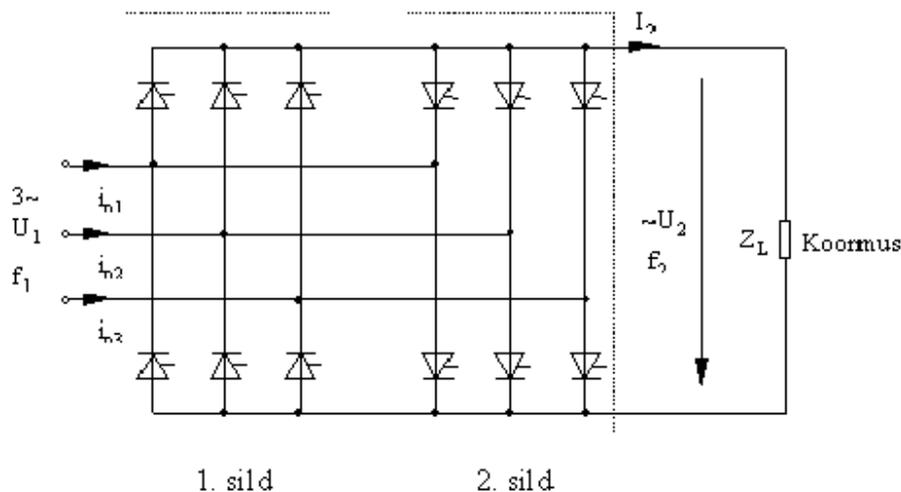
Figure 4.31. Circuit diagram of the Single-phase cycloconverter
