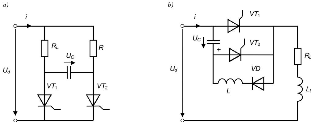
Figure 4.4. Commutation circuits of a thyristors in a direct current circuit
