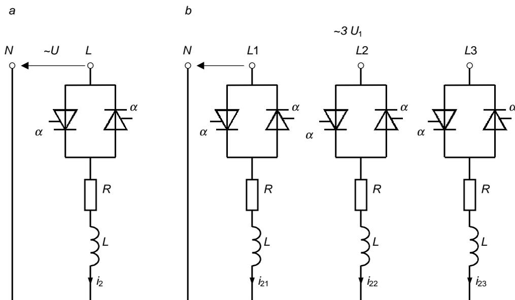
Figure 4.15. Alternating current controllers: a) single-phase controller, b) three-phase controller
