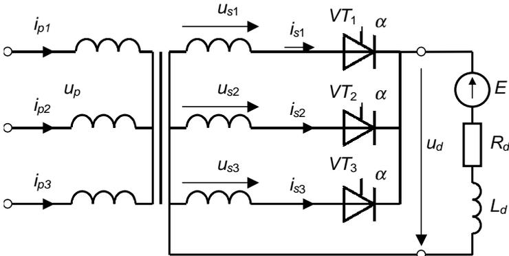
Figure 4.10 Three-phase mid-point rectifier (M3)
