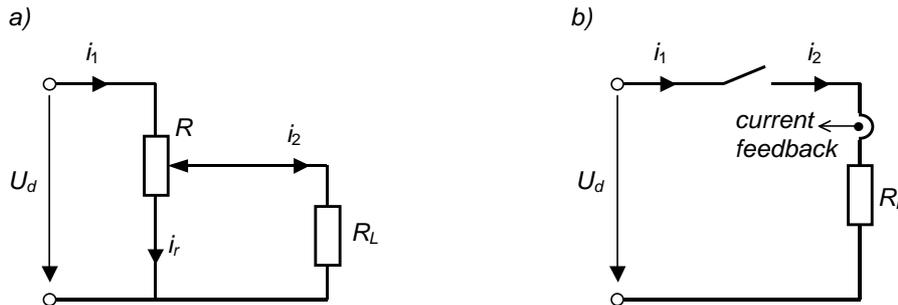
Figure 4.1. Control of the load voltage and current using a) resistor, b) switch
