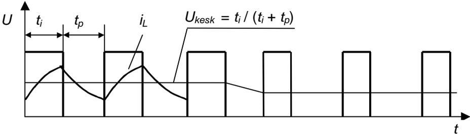
Figure 4.2. Pulse with modulation principle
